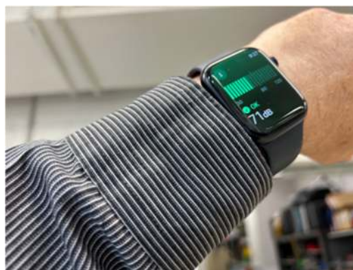
Figure 1 General Air Extraction Noise level - 71 dBA
